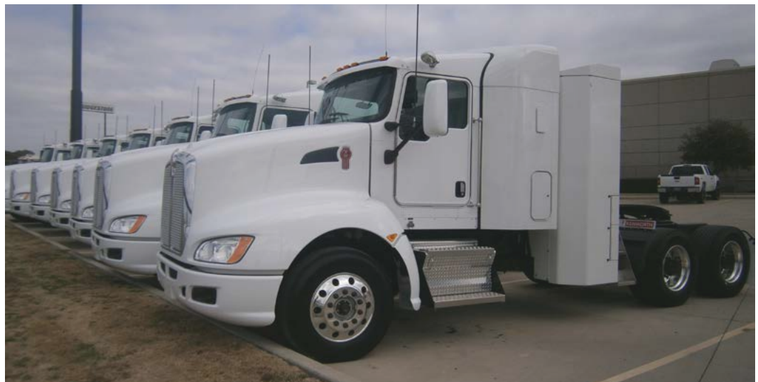
Right Fleet of 11.9L Kenworth trucks with a 125 DGE back-of-cab CNG tank system
